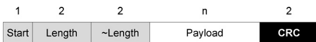
Fig. 4. SSI/UART message format. Start byte indicating beginning of message is 0×FE. Length and ~Length are length and bitwise not of length of message payload with optional CRC.
